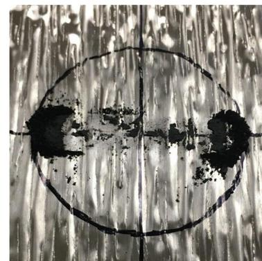
Figure 4: Medium Magnet Wear Debris Pattern
