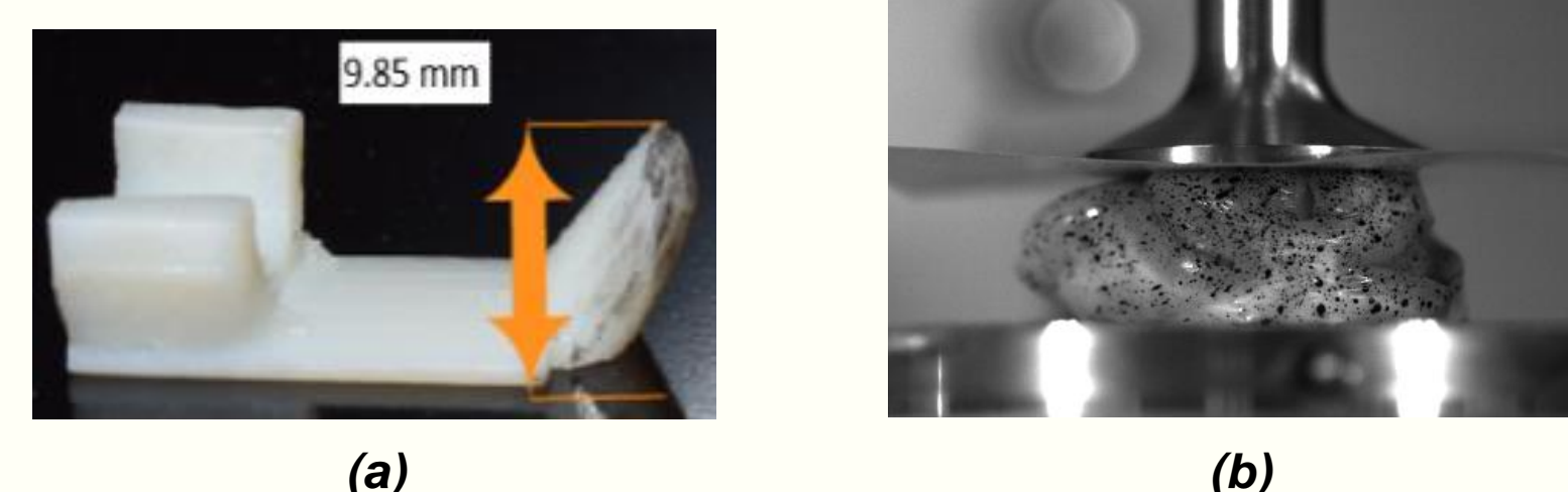
Figure 3: (a) Airbrush Attachment and (b) Airbrush Speckle Pattern on Brain
